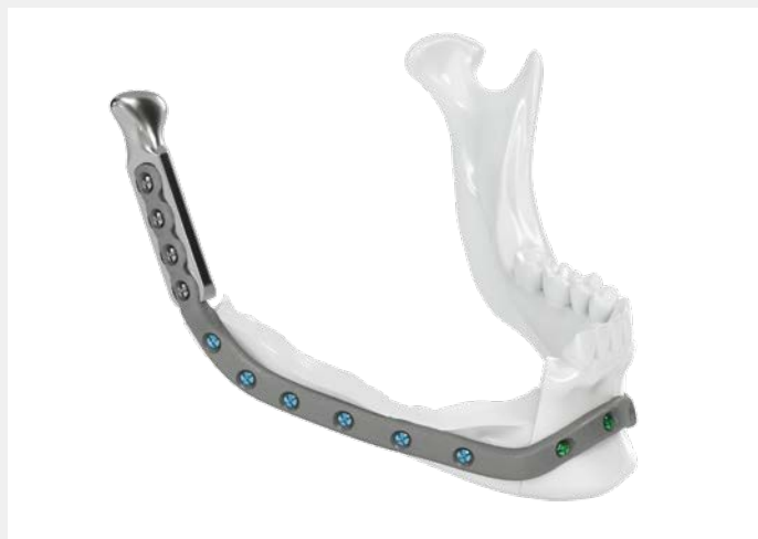
Mandibular reconstruction without transplant planning Restoration with additive-manufactured IPS® plate and temporary condyle implant. Fixed with locking and standard screws.
