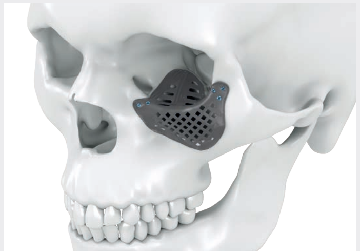
Orbital reconstruction with additively manufactured titanium implant including zygoma mesh. Fixation with standard screws 1.5 mm.
